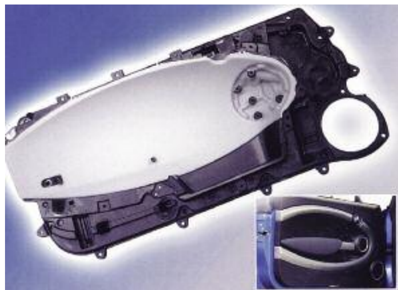
The plastic door modules for the new BMW Mini are made from custom-engineered TechnoCompound glass-fibre reinforced polypropylene
